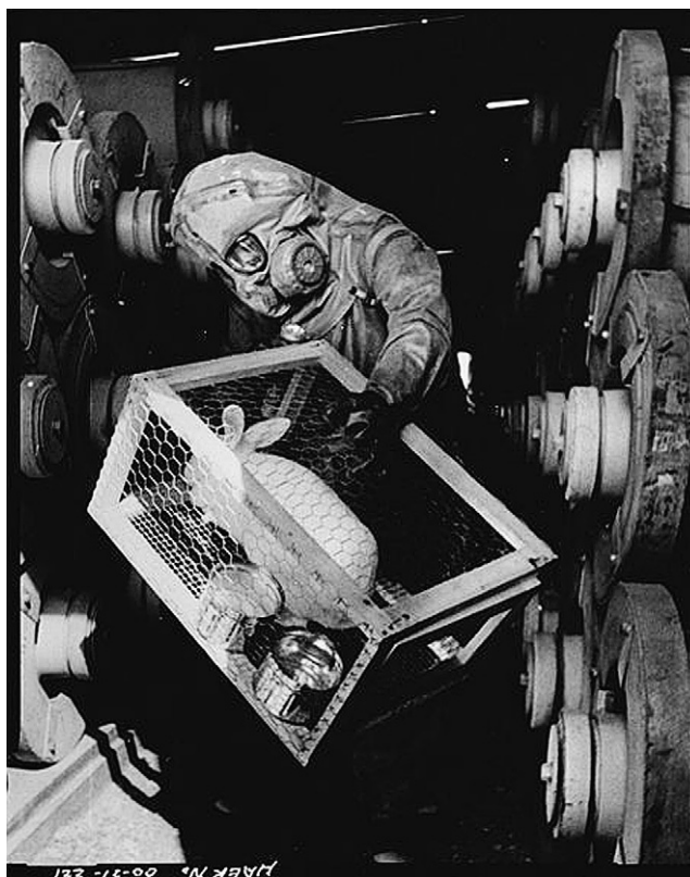
FIGURE 2.9. Testing for leaks at Sarin production plant, 1970. Source: Library of Congress ( http://memory.loc.gov/pnp/habshaer/co/co0100/co0168/photos/316333pr.jpg ).
