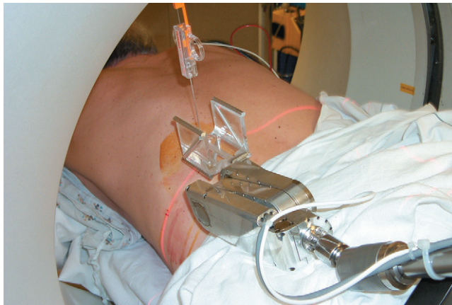
FIGURE 1-3 The z-PAKY being tested under computed tomography (CT) guidance. (Courtesy of the Urobotics Laboratory, Johns Hopkins, Baltimore, MD.)
