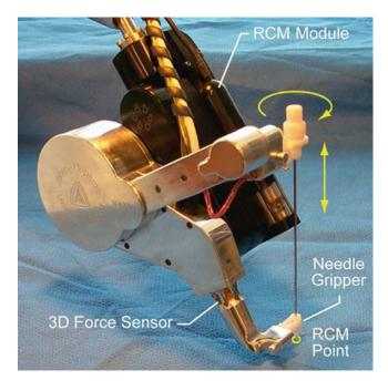
Fig. 1.2 Revolving needle driver on the AcuBot robot
