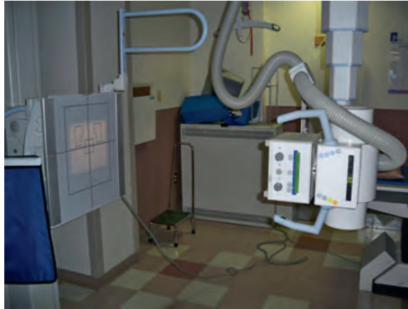
Figure 1-2. Typical DR unit with x-ray tube located on right and anti-scatter grid and flat panel detector located on left.
