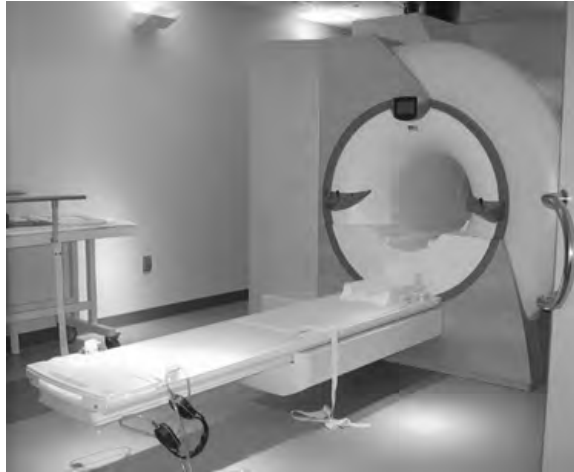
Figure 2-4. Typical MRI scanner with MRI gantry (which contains superconducting magnet) and patient table.
