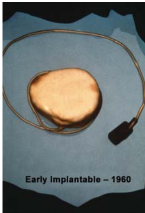
Figure 1.3 History – First “permanent” implantable pacemaker and bipolar Hunter–Roth lead (1958). (Source: Reproduced with permission of Medtronic, Inc.)
