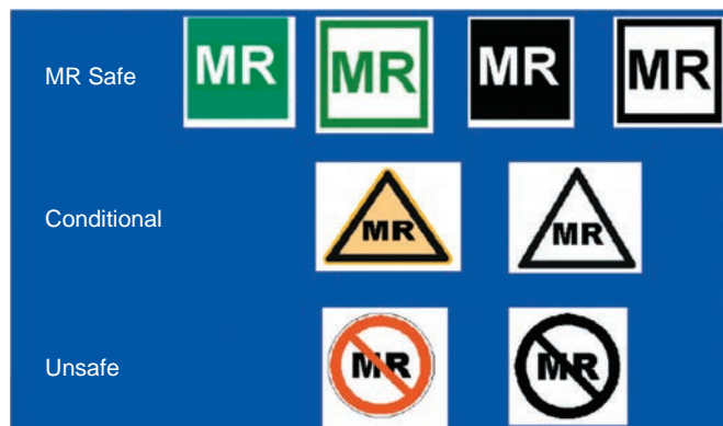
Figure 2.3. International magnetic resonance safety labeling icons. US FDA labeling criteria (developed by American Society for Testing and Materials International) for portable objects (e.g., medical devices, implants, medical equipment, oxygen tanks, housekeeping equipment, and tools) that may or may not enter the MR environment. Square/green “MR safe” labels correspond to objects that are totally nonreactive, triangular/yellow labels correspond to objects with “MR conditional” status, and round/red labels identify an object as being “MR unsafe.” The use of the new labeling convention has been adopted by the FDA and applied to items prospectively (but not retrospectively), beginning approximately in August 2005. (From ASTM International. Standard practice for marking medical devices and other items for safety in the magnetic resonance environment [designation F203-5], West Conshohocken, PA: ASTM International; 2005.)
