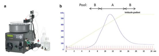
Fig. 5 (a) ÄKTA Prime system used for elution and fraction recovery; (b) Chromatogram of human IL-6R purification on a nickel chromatography resin, with fractions pooled to obtain a high (a) and a low (b) concentration batch
