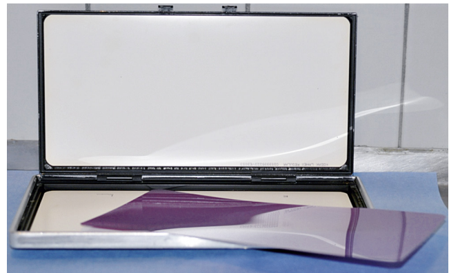
Figure 2-4 An opened panoramic cassette (15 × 30 mm) with intensifying screens on both sides (white surfaces) and analog film (blue-purple). A similar cassette, but without intensifying screens, is used for phosphor storage plates.
