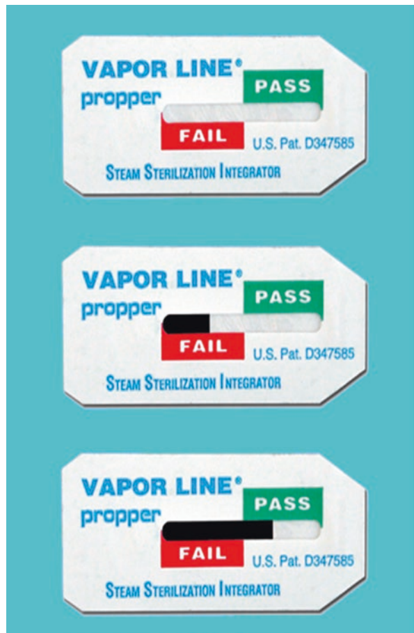
Photo 2.1 Example of a chemical multiparameter integrator (courtesy of Vapor Line)
