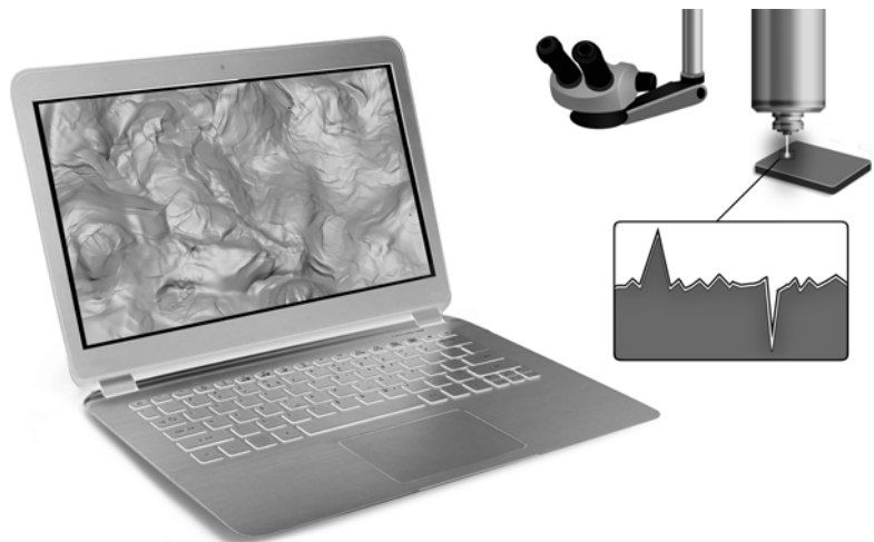
Fig. 1.2 A drawing of an optical profiler. Due to the noncontact technique, the horizontal resolution is increased. The light beam can follow the irregularities quite well (Figure produced by Braian Development AB, Malmö, Sweden)
